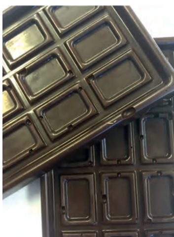
Figure 2: Incorrect viscosity may result in holes in the chocolate.
